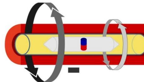
coaxial cylinder measuring system
