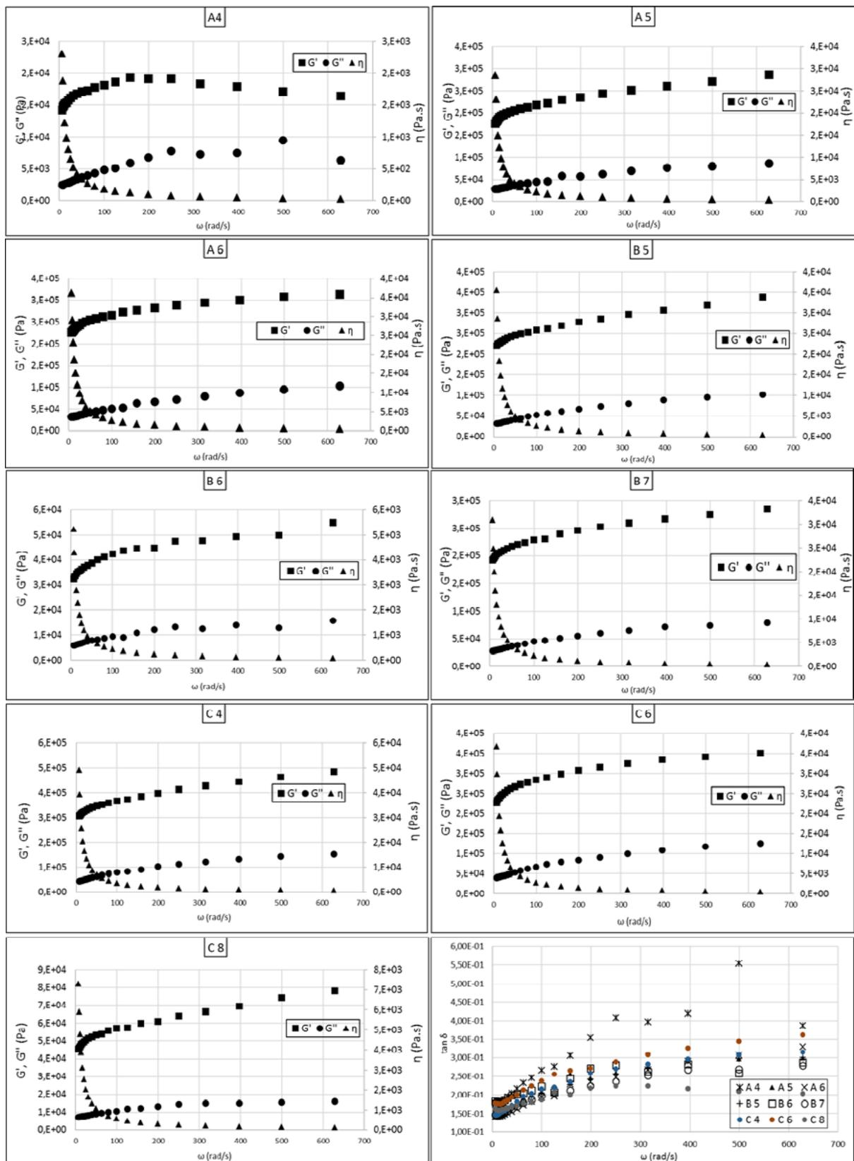
Figure 1 - Viscoelastic properties of watery oleogels containing 5% wax
