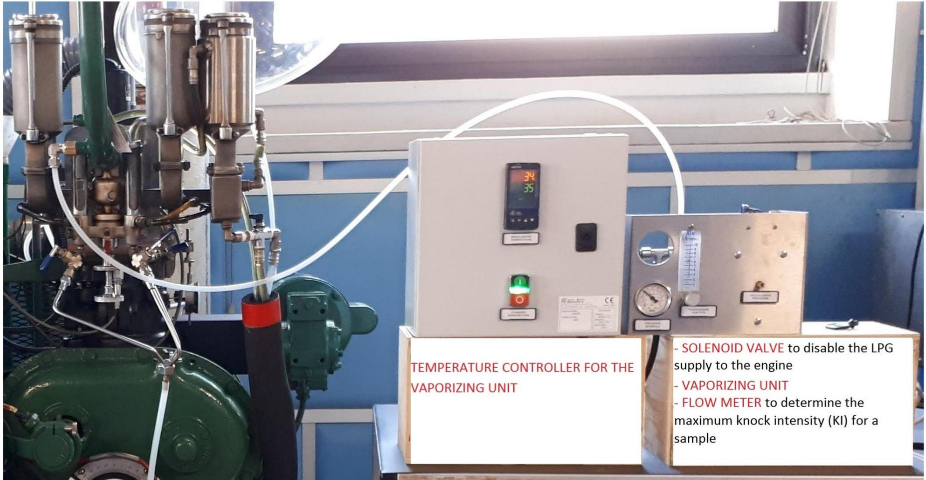
The fuel is drawn from the cylinder as a liquid, vaporized and maintained at a constant temperature, then introduced into the air stream at constant pressure through a connection on the standard carburetor inlet elbow, upstream of the venturi
