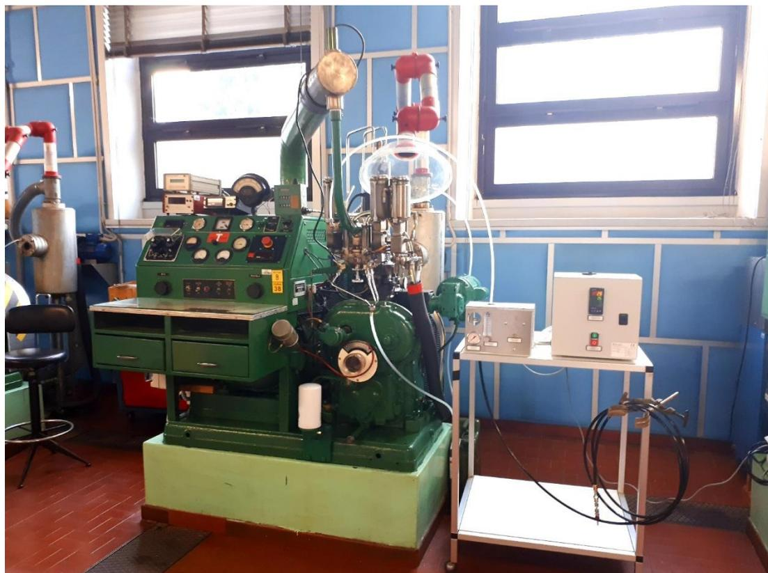
CFR engine equipped with LPG kit
