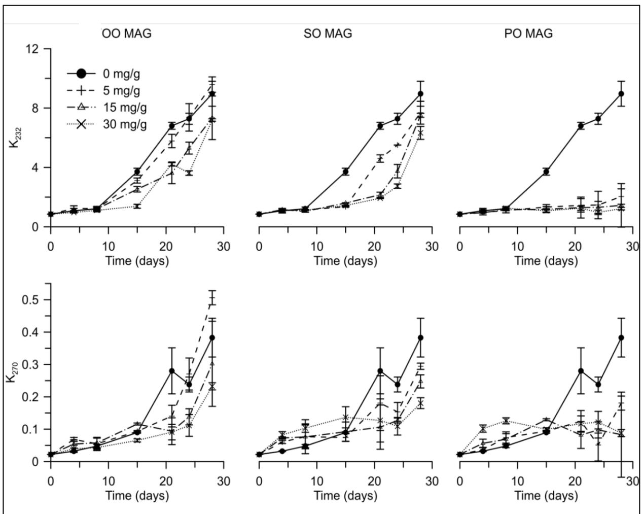
**Figure 2** - Determination of spectrophotometric constants ( $K_{232}$ ,  $K_{270}$ ) in purified olive oil and in the same added with 0.5%, 1.5%, and 3% of monoacylglycerols (MAG-5 mg/g, MAG-15 mg/g, MAG-30 mg/g) of olive oil (OO), soybean oil (SO), and palm oil (PO) during the oven test at 60°C.
