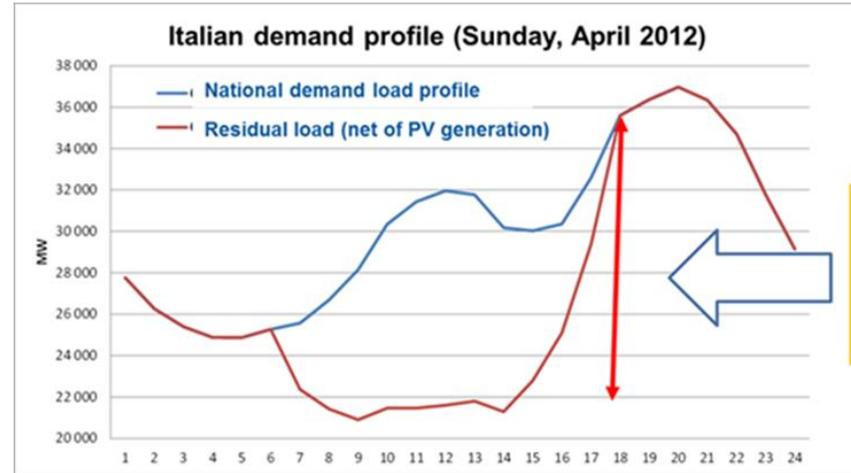
14 GW of load ramp in the evening to be covered by dispatchable generation and import
